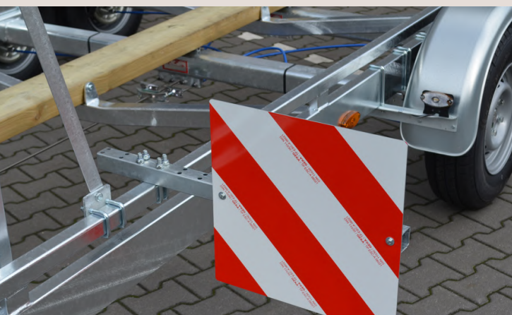
Width marker boards
