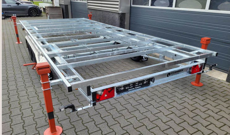
Support legs for deck (4x 3000 kg)
