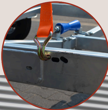
Holes for Strap Attachment
