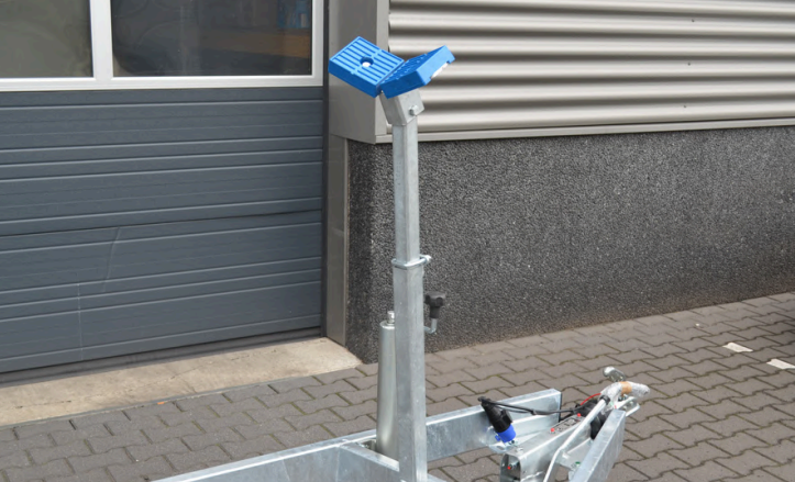
Winch support with catchment mouth
