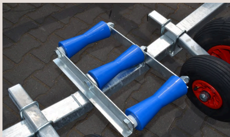
Keel roller tilting system
