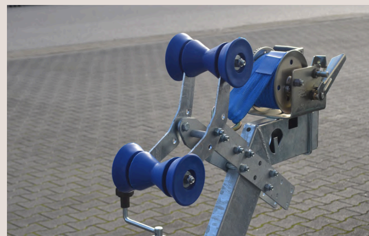
Double roller catch jaw
